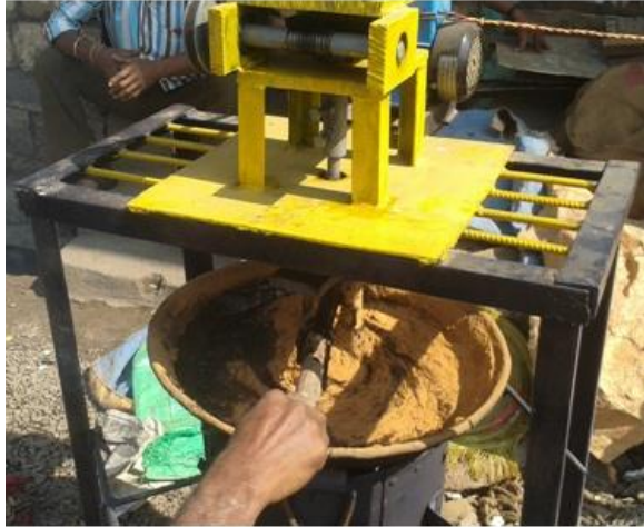
Fig. 3.1. Early trials of planetary stirrer
