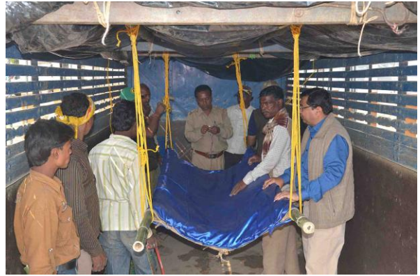
Fig-2: Hanged rescue stretcher on a truck.
