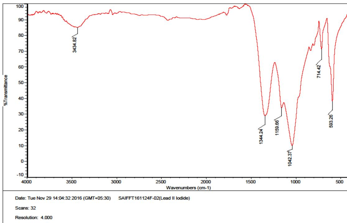
**Figure.10.** FTIR spectra of lead II iodide nanoparticles.
