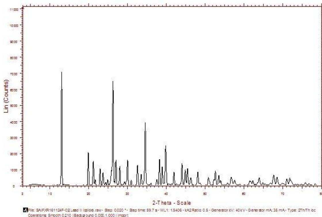
**Figure .1.** XRD pattern of lead II iodide nanoparticles.
