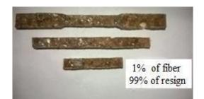
(b) Specimen at 1% fiber 99% resin
