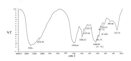
Figure 1 - FTIR spectrum of in house Dextran
