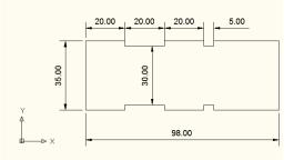
FIGURE 2. WORK PIECE GEOMETRY
