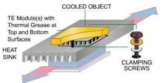
TE Module Installation Using the Clamping Method
