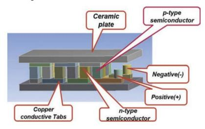
Waste heat can be supplied to top ceramic plate of thermoelectric generators. This waste heat comes from industry and infrastructure-heating activities, automobile engines exhaust and geothermal.
