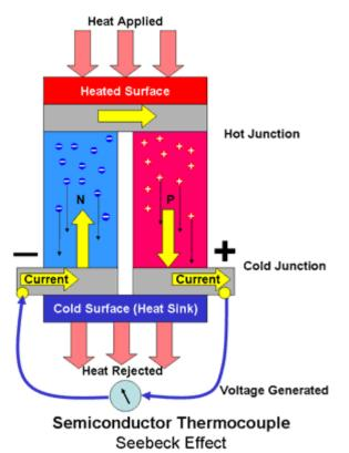
Thermocouple is the device to measure temperatures. It consists of at least two metals joined to form two junctions. As shown in the picture metals are cold at one end and hot at another end. When two different metals are combined with different temperatures the current is generated between the two junctions. Thermocouple is the device to measure temperatures. It consists of at least two metals joined to form two junctions. As shown in the picture metals
