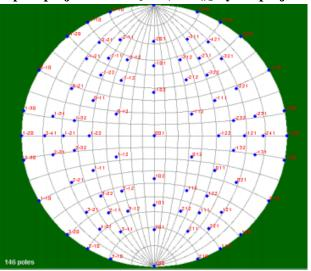
Figure 8: Stereographic projection of  $K_3Na$  ( $CrO_4$ )<sub>2</sub>crystal projected at 001 direction Table 2: Values of measured and computed interfacial angles of  $K_3Na$  ( $CrO_4$ )<sub>2</sub> crystal.
