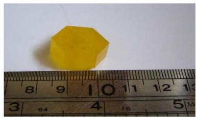
Figure 3: Photograph of the grown K<sub>3</sub>Na (CrO<sub>4</sub>)<sub>2</sub> crystal.
