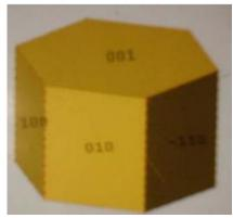
Figure 4: Morphology of K<sub>3</sub>Na (CrO<sub>4</sub>)<sub>2</sub> Crystal.
