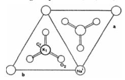
Figure 2: View along the c - axis of K<sub>3</sub>Na(CrO<sub>4</sub>)<sub>2</sub> crystal.
