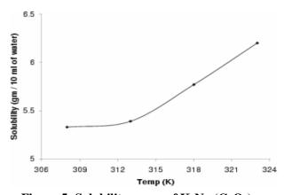
Figure 5: Solubility curve of K<sub>3</sub>Na (CrO<sub>4</sub>)<sub>2</sub>.
