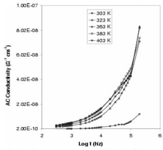
Figure 10: Variation of measured ac conductivity with frequency along c-axis
