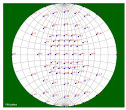
Figure 7: Stereographic projection of K<sub>3</sub>Na (CrO<sub>4</sub>)<sub>2</sub>crystal projected at 100 direction
