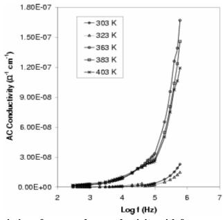
Figure 9: Variation of measured ac conductivity with frequency along a-axis.
