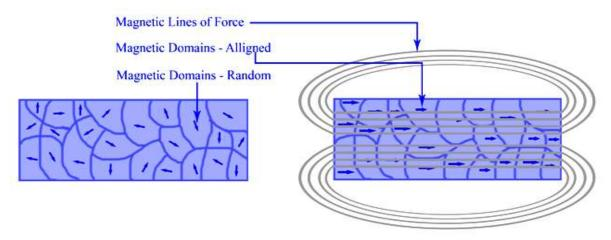
: Ferromagnetism (a) nonmagnatized material and (2) Magnetized material with corresponding magnetic fields shown.
