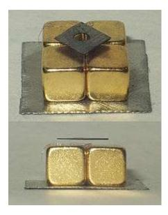
: Levitating pyrolytic carbon: A small (~6 mm) piece of pyrolytic graphite levitating over a permanent neodymium magnet array (5 mm cubes on a piece of steel). Note that the poles of the magnets are aligned vertically and alternate (two with north facing up, and two with south facing up, diagonally).
