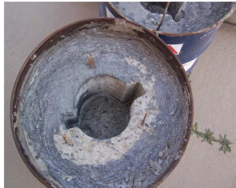
Fig.(2) 200 L drum for the prefabricated cask contain the dismantled CO-60 or Cs-137 sources[1].
