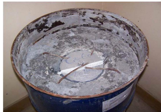
Fig.(4) 200L drum contains the prefabricated Cask contains the dismantled Co 60 or Cs 137
