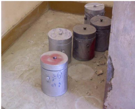
Fig. (1) Prefabricated casks contain the dismantled Co-60 or Cs-137 sources [1]. or
