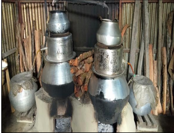
Distillation Setup for extraction of alcohol
