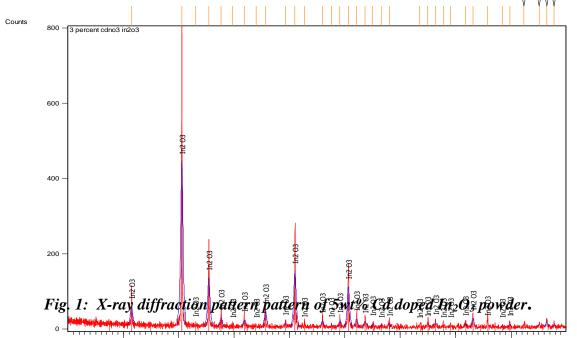
From Debey Scherrer's Formula (i.e.  $D = k \Lambda \beta \cos \theta$ ), where  $\Lambda$  is the wavelength of X-ray radiation, k is constant, 20 is the diffraction angle,  $\beta$  is the full width at half maximum., average crystalline size of Cd doped In<sub>2</sub>O<sub>3</sub> is 20.17 nm and crystallinity of Cd doped In<sub>2</sub>O<sub>3</sub> powder is 83.17 percent.
