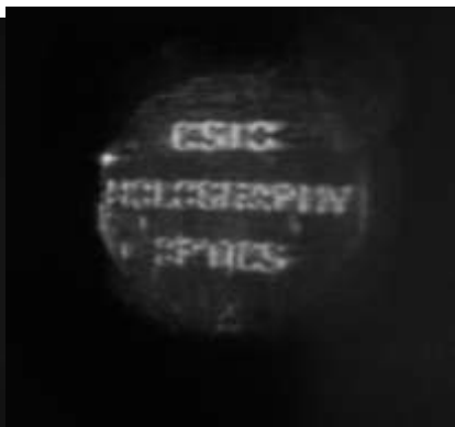
Figure 4- An optical image processed with modified schlieren system
