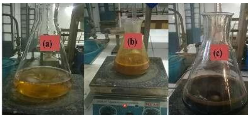
Figure 9: (a) Ficus hispida Linn.f. leaf extract (b) \text{FeCl}_3 \cdot 6 \text{H}_2\text{O} and \text{FeSO}_4 \cdot 7\text{H}_2\text{O} added in a 2:1 ratio to the extract (c) \text{NH}_3 base added to the solution mixture to create Ficus hispida Linn.f. leaf mediated \text{Fe}_3\text{O}_4 NPs
