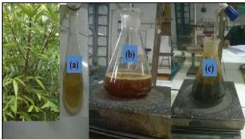
Figure 8: (a) ZA DC. leaf extract (inset plant picture) (b) \text{FeCl}_3 \cdot 6 \text{H}_2\text{O} and \text{FeSO}_4 \cdot 7\text{H}_2\text{O} in 2:1 ratio added to the extract (c) \text{NH}_3 base added to the solution mixture to create ZA DC. leaf mediated \text{Fe}_3\text{O}_4 NPs at 80 °C
