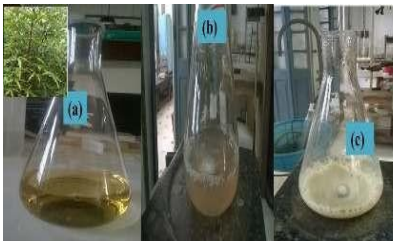
Figure 6: (a) Leaf extract of ZA DC. (inset plant image) (b) Solution mixture created after addition of \text{Zn}(\text{CH}_3\text{COO})_2 \cdot 2\text{H}_2\text{O} to the extract (c) Leaf mediated ZnO NPs formed after addition of NaOH base to the solution mixture at 70^\circ\text{C}
