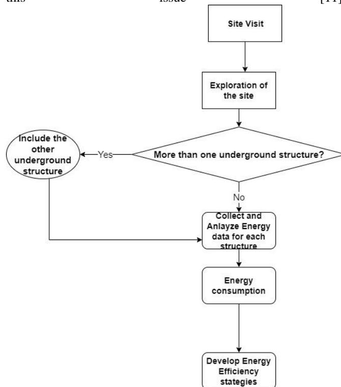
Fig i: Analysis process of underground space energy efficiency
