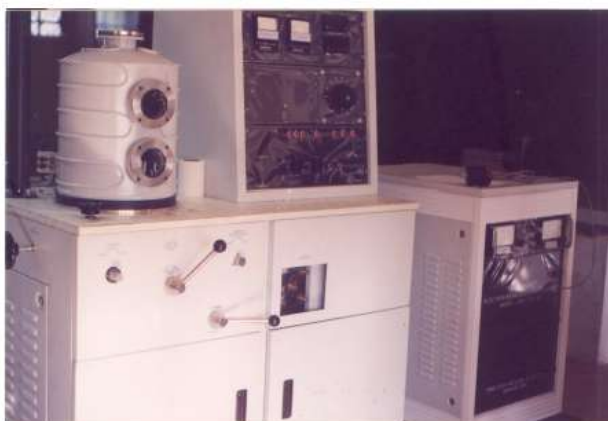
Figure 2 Photograph of coating unit and electron beam power supply
