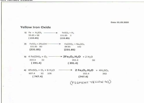
Hence before reaction goes to final stage of filtration, we have decided to apply surface treatment to improve final products dispersibility. The final slurry of pigment yellow 42 or simple synthetic Iron
