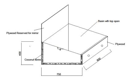
Fig 1 Cross Section of the Solar Still under Construction
