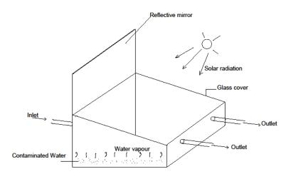
Fig 2 Operation of Solar Still
