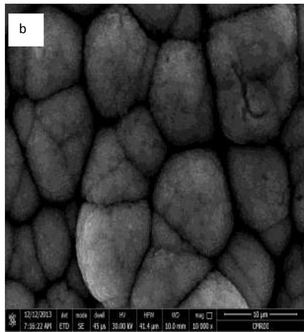
Fig.2 (a, b): Scanning electron microscope of as plated electroless (a) Ni-Sn-P and Ni-Sn-P after blackening.
