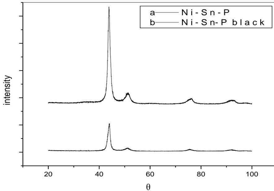
Figs.1 (a,b) show X-ray diffraction patterns of aluminum substrate, Ni-Sn-P and black Ni-Sn-P.
