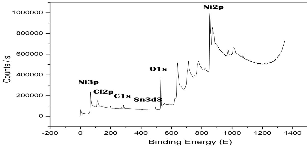
Fig.3: XPS wide scan spectrum of black Ni-Sn-P.
