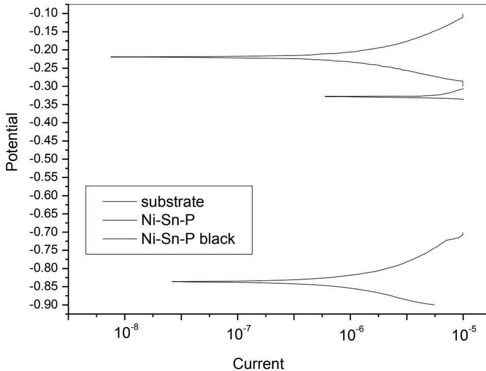
Fig.(5) shows potentiodynamic curves of (a) the substrate , (b) as deposited electroless Ni-Sn-P coat and (c) black coat Ni-Sn-P in 3.5% sodium chloride solution.
