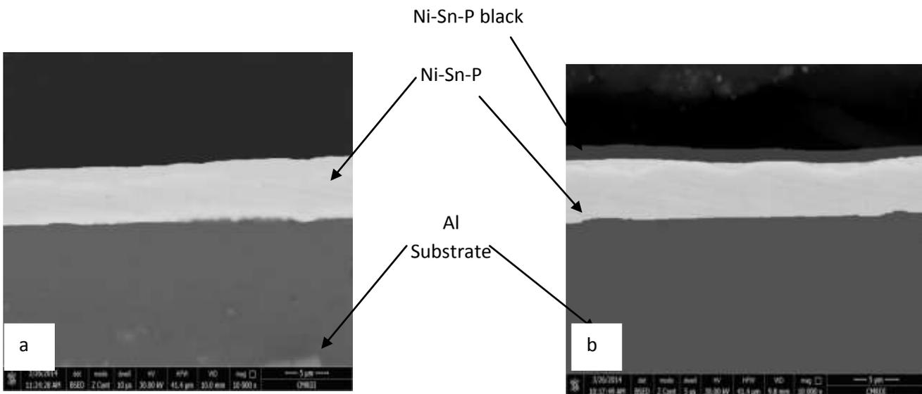
Fig.4 (a, b) Cross section of Ni-Sn-P and Ni-Sn-P black layers.
