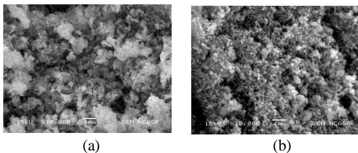
**Figure 3: SEM micrograph of (a)  $\text{Ni}_{0.4}\text{Zn}_{0.6}\text{Fe}_2\text{O}_4$  and (b)  $\text{Ni}_{0.8}\text{Zn}_{0.2}\text{Fe}_2\text{O}_4$ .**
