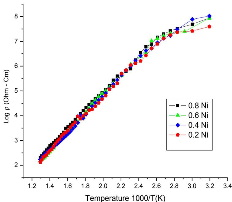
**Figure 4: Variation of resistivity (log $\rho$ ) with 1000/T (K) for  $\text{Ni}_x\text{Zn}_{(1-x)}\text{Fe}_2\text{O}_4$  samples.**
