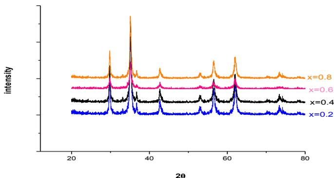
**Figure 1: XRD pattern of  $\text{Ni}_x\text{Zn}_{(1-x)}\text{Fe}_2\text{O}_4$  samples**
