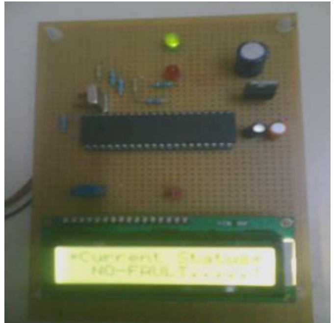
Fig. 12 Display Unit under No-Fault condition
