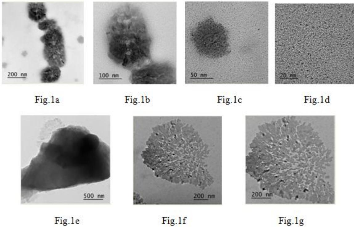
**Fig.1** TEM images of magnesium carbonate nanoparticles
