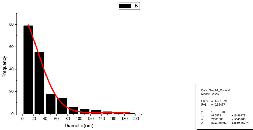
**Fig.2.** The size distribution histogram for magnesium carbonate nanoparticles
