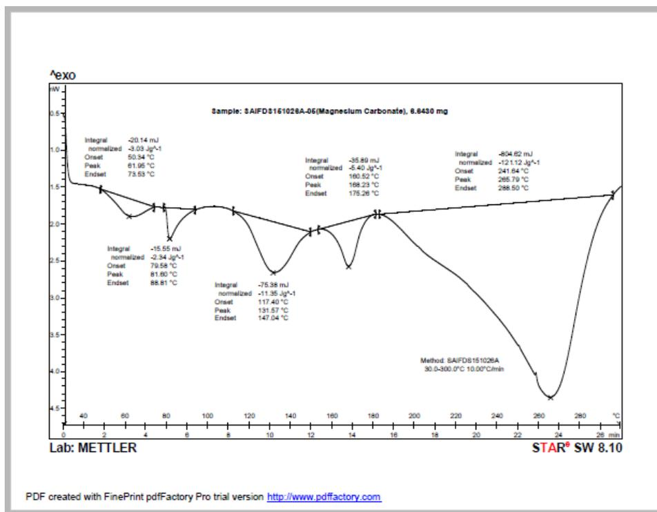
**Fig.4.** DSC curve of magnesium carbonate nanoparticles
