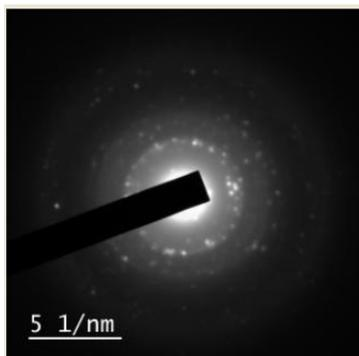
**Fig.3.** The SAED pattern of magnesium carbonate nanoparticles
