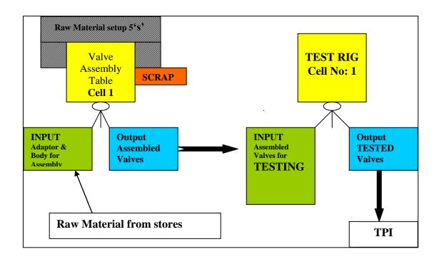
**AFTER Standard Work Kaizen-** Streamlined Work Flow of Valve Assembly Process.
