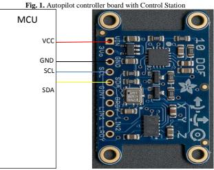
Fig.2 DOF –IMU Sensor Wiring
