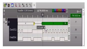
Fig.5 Timing Plot I2C communication shown in logical analyzer
