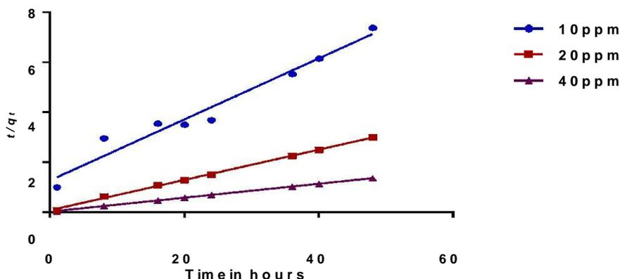
**Figure-9: Pseudo Second order kinetic model for Adsorption of alizarin red dye by immobilized *Saccharomyces cerevisiae* beads**
