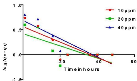
**Figure-7: Pseudo first order kinetic model for Adsorption of alizarin red dye by immobilized *Saccharomyces cerevisiae* beads**
