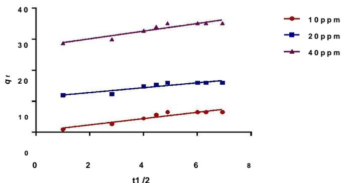
**Figure-13: Intraparticle Diffusion model for Adsorption of alizarin red dye by immobilized *Saccharomyces cerevisiae* beads**
