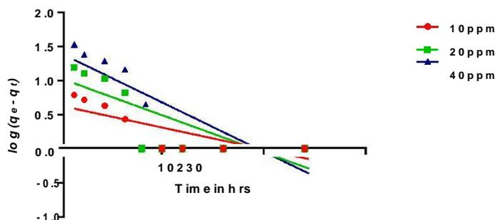
**Figure-8: Pseudo first order kinetic model for Adsorption of alizarin red dye by Calcium alginate beads**
