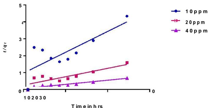
**Figure-10: Pseudo Second order kinetic model for Adsorption of alizarin red dye by Ca-alginate beads**
