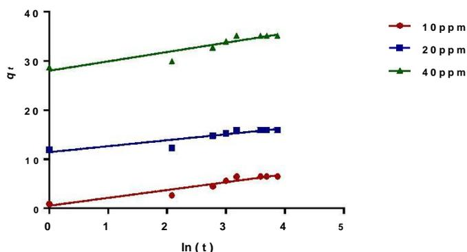
**Figure-11: Elovich Model for Adsorption of alizarin red dye by immobilized *Saccharomyces cerevisiae* beads**
