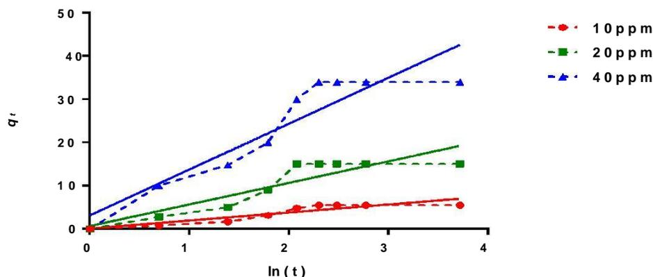
**Figure-12: Elovich Model for Adsorption of alizarin red dye by Ca-alginate beads**
