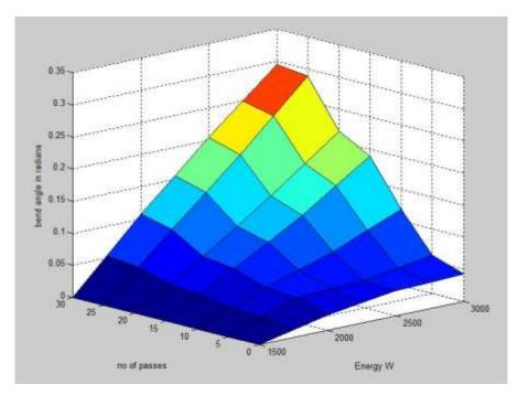
Figure 2: Effect of Energy and Number of Passes on Bending Angle 4. ESTIMATION OF NN MODEL
