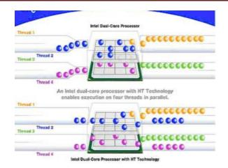
While Hyper threaded CPUs appear as two logical processors to most operating systems, they are not comparable with true dual-core CPUs since each parallel pair of threads being worked on share the same execution pipeline and same set of L1 and L2 cache memory. Essentially, Hyper threading is smoke-and-mirrors multitasking, since a single Hyper threaded processor cannot actually perform two identical actions at the same time.
