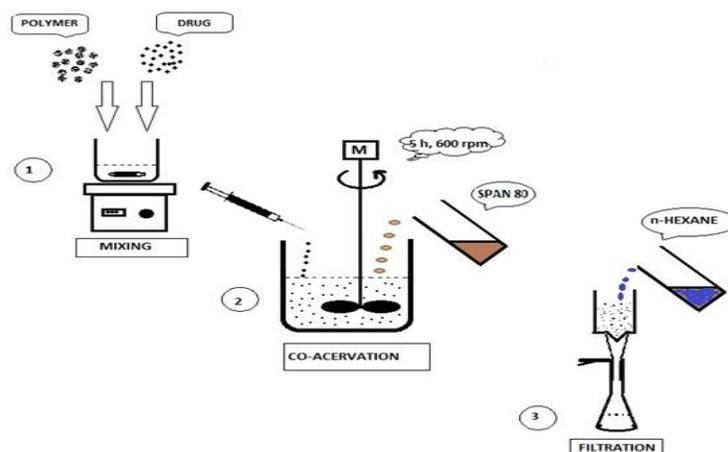
Figure 1. Flow chart for preparation of Microspheres
