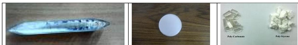
Figure 1.(a) Ingot after zone refining (b) Silicon rubber composite of cadmium iodide (c) Matrix materials polycarbonate and polystyrene
