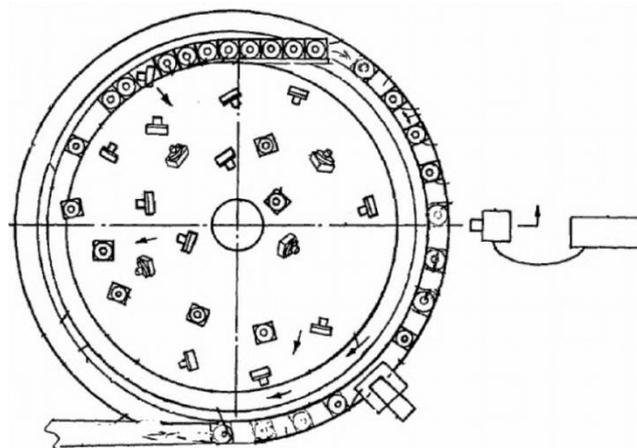
Figure 10. Second Transparent Track with the Vision Inspection System [10]
