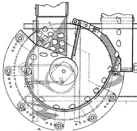
Figure 5. Single Conical Rotating Surface for Uneven Objects Orientation[5]
