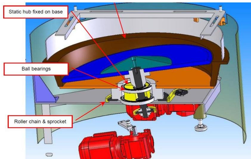
Figure 11. Disc Shaft Pass through the Fix Static Hub and Bowl Hub Mounted On Static Hub [2]
