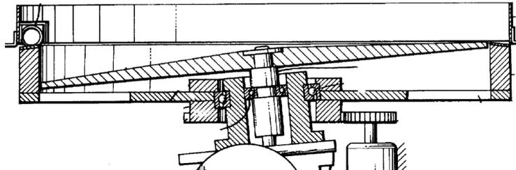
Figure 3. Centrifugal Feeder with Non- Planner Disc and Rim Surface [3]
