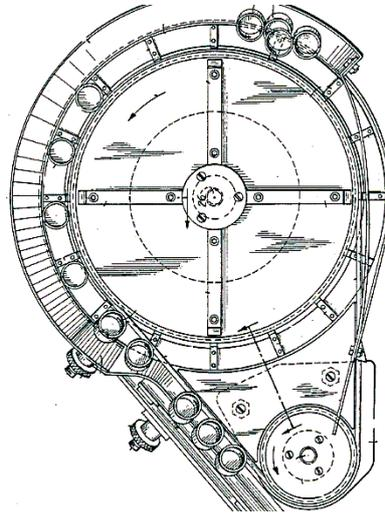
Figure 6. Rotary Feeder with Single Rotating Disc Which Rotate By Pulley and O-Ring [6]
