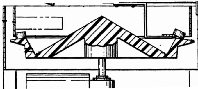
Figure 7. Rotary Feeder with Conical Surface with Tangential Flange [7]
