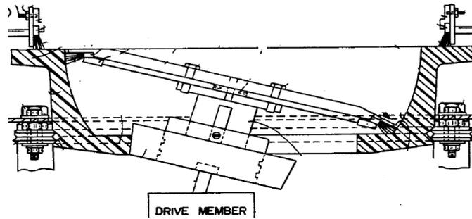
Figure 8. Disc Extension by Brush for Cover the Gap between Disc and Bowl [8]
