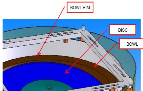
Figure 1. Main components of centrifugal feeder [2]
