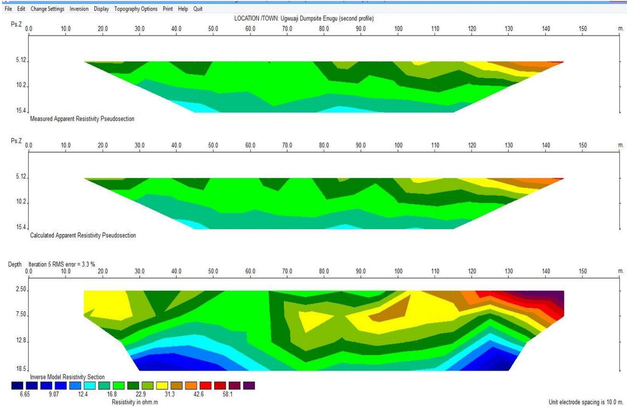
Figure 7: Electrical resistivity tomography – profile 2.
