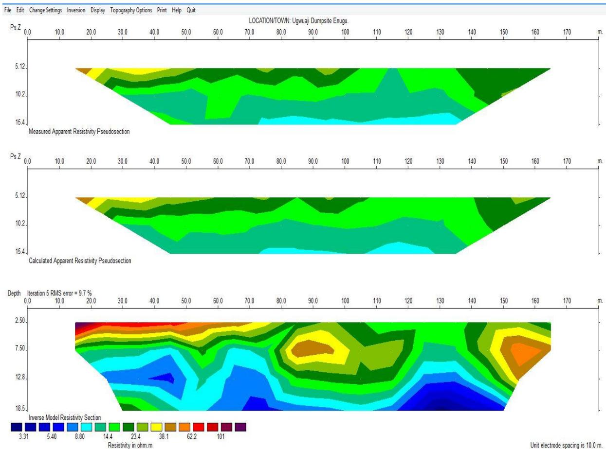
Figure 6: Electrical resistivity tomography – profile 1.
