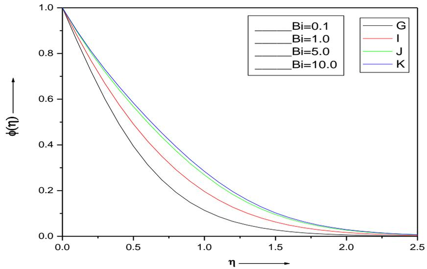
**Fig. 9. Effect of  $Bi$  on concentration profiles when  $Nt = Nb = 0.1, Pr = Le = Ec = 5$ .**
