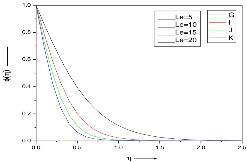
**Fig. 8. Effect of  $Le$  on concentration profiles when  $Nt = Nb = 0.1, Pr = 5, Ec = 5, Bi = 0.1$ .**
