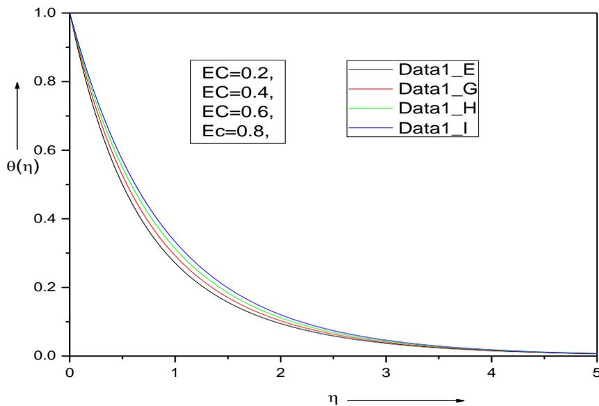
**Fig. 6 Effect of Eckert Number on Temperature profile for different values of**
