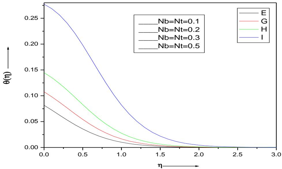
**Fig. 1. Effect of  $Nt$  and  $Nb$  on temperature profiles when  $Le = 5, Pr = 5, Ec = 5, Bi = 0.1, M = 2.$**
