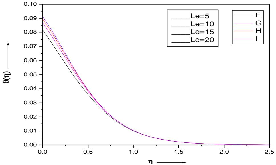
**Fig. 2. Effect of  $Le$  on temperature profiles when  $Nt = Nb = 0.1, Pr = 5, EC = 5, Bi = 0.1, M = 2.$**
