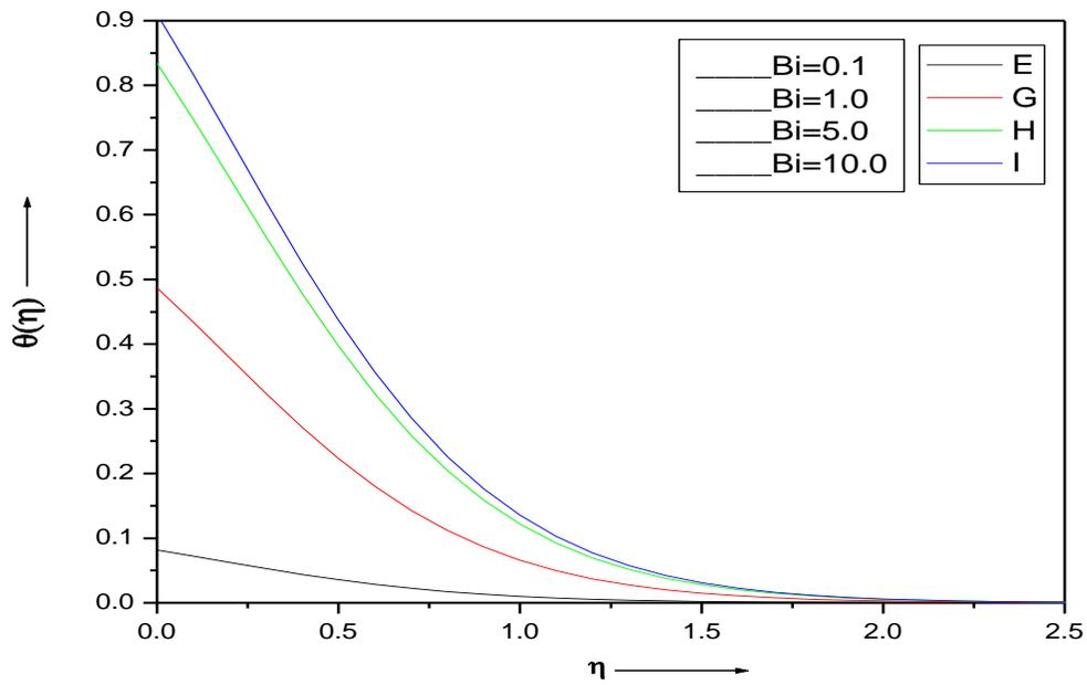
**Fig. 3. Effect of  $Bi$  on temperature profiles when**
