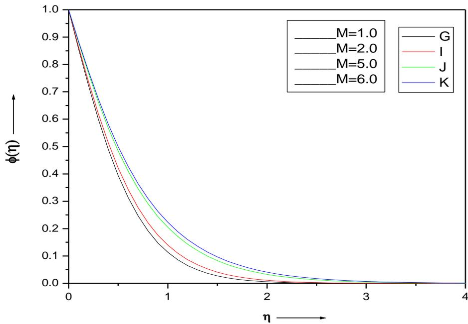
**Fig. 10. Effect of  $M$  on concentration profiles when**
