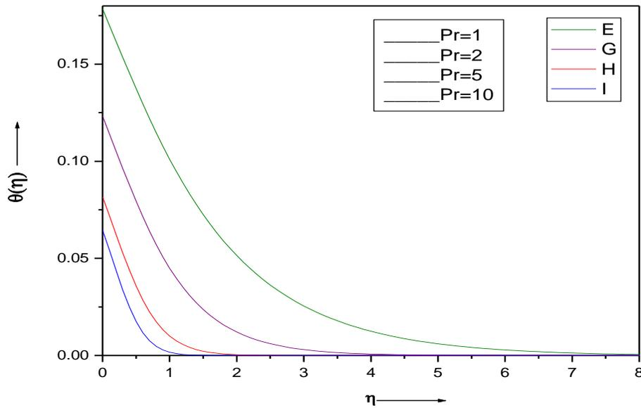
**Fig. 4. Effect of  $Pr$  on temperature profiles when**
