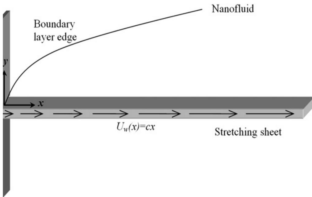
**Fig A: boundary layer flow over a stretching sheet.**
