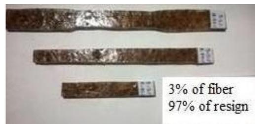
(d) Specimen at 3% of fiber 97% resin
