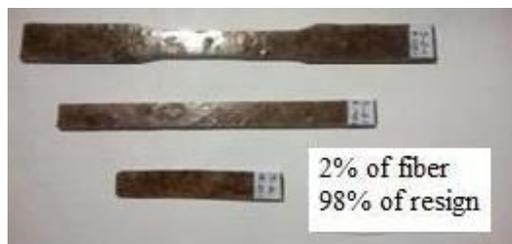
(c) Specimen at 2% fiber 98% resin
