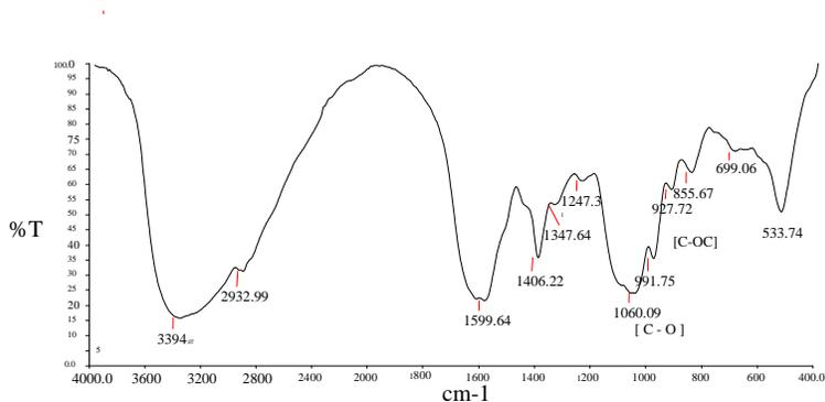
Figure 1 - FTIR spectrum of in house Dextran
