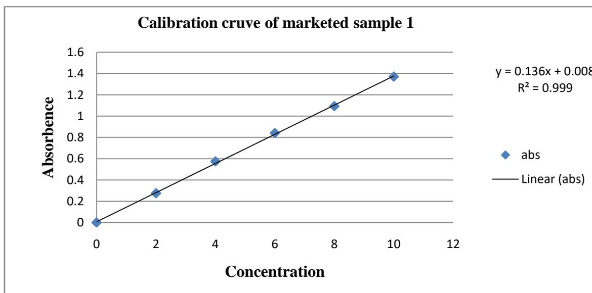
Figure No: 11 Linearity curve of sample 1 Glycyrrhetic acid
