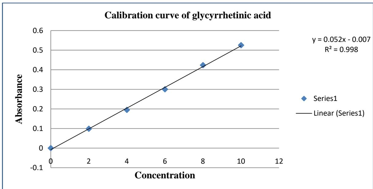
Figure No: 10 Linearity curve of standard Glycyrrhetic acid
