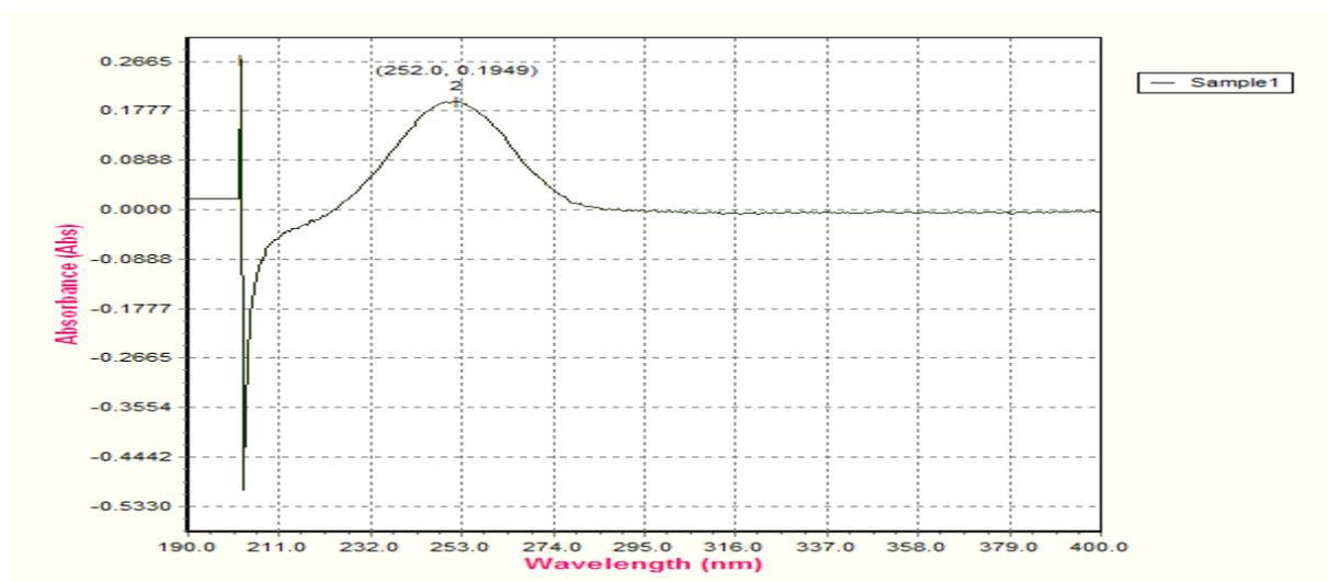
Figure no: 4 Absorption curve of standard Glycyrrhetic acid
