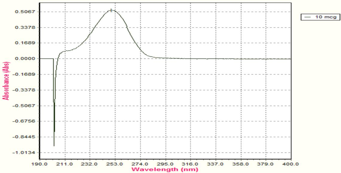
Figure no: 8 Absorption curve of standard Glycyrrhetic acid
