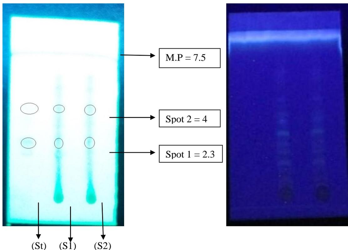
a. Short wavelength (254nm) b. Under long wavelength (365nm)
