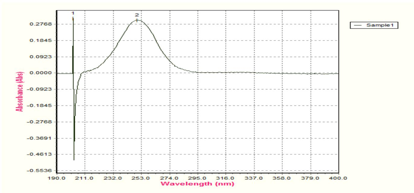
Figure no: 6 Absorption curve of standard Glycyrrhetic acid
