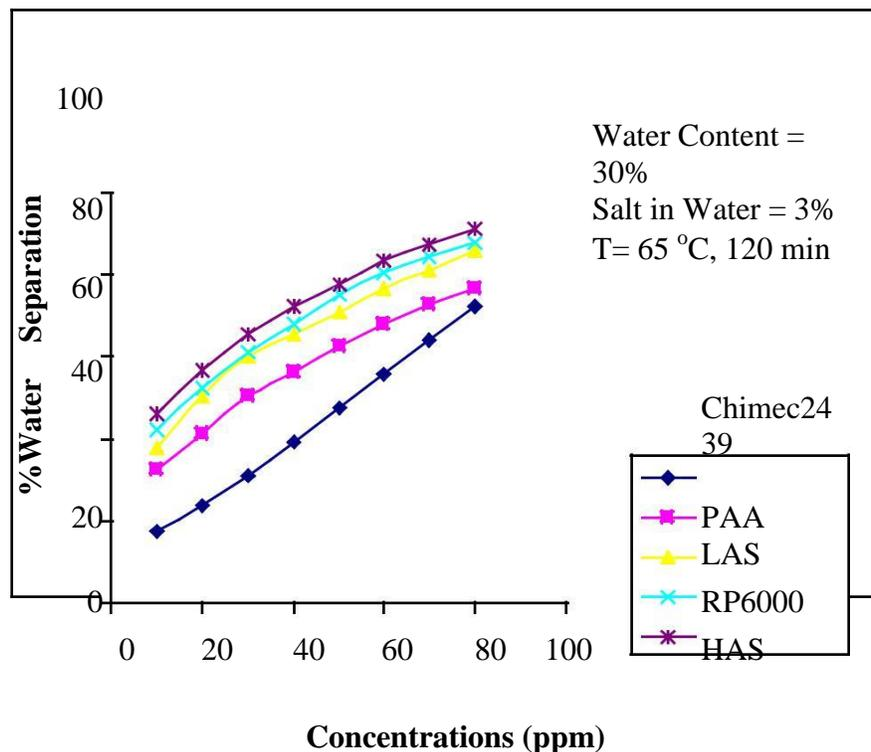
Figure 1: Effect of Concentrations on Water Separation for RP6000, Chimec2439, PAA, LAS and HAS at 120 minutes
