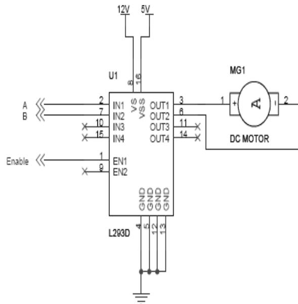
Fig.3 Schematic for interfacing a DC motor using L293D
