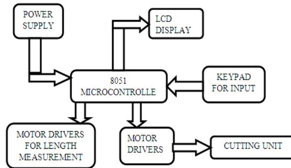
Fig.1 Block diagram of automatic wire cutting machine
