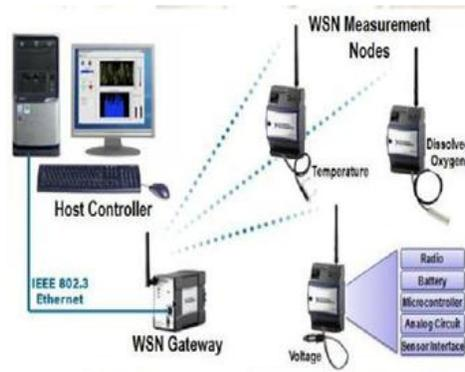
**Figure 1: Common Wireless Sensor Network Architecture**
