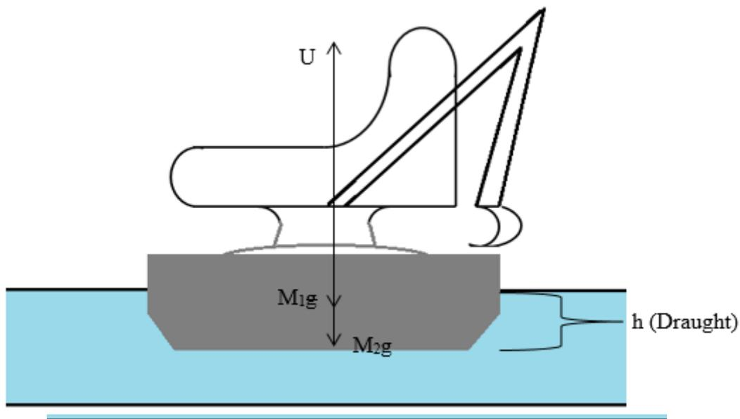
**Figure 01:** Force Application of the Barge and Excavator
