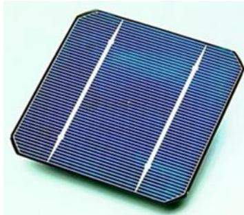
Solar cell consists of a n-type semiconductor layer and p-type semiconductor layer. The two layers are combined to form a p-n junction. Anti-reflection coating is used to avoid the loss of incident light energy due to reflection at the surface.
