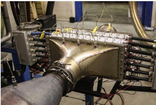
TEG are used to boost efficiency by converting the waste heat into electricity. In the fig shown to recapture the heat energy generators are used and exhausted by diesel vehicles.
