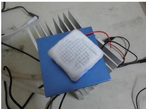
Peltier effect use in thermoelectric applications. Peltier module has been used in many
