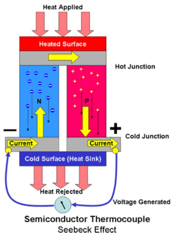
Thermocouple is the device to measure temperatures. It consists of at least two metals joined to form two junctions. As shown in the picture metals are cold at one end and hot at another end. When two different metals are combined with different temperatures the current is generated between the two junctions. Thermocouple is the device to measure temperatures. It consists of at least two metals joined to form two junctions. As shown in the picture metals
