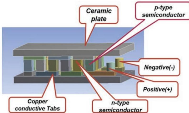
Waste heat can be supplied to top ceramic plate of thermoelectric generators. This waste heat comes from industry and infrastructure-heating activities, automobile engines exhaust and geothermal.
