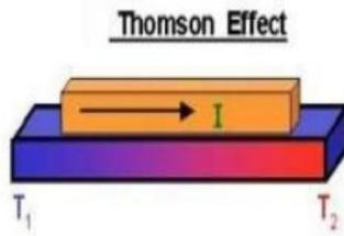
Small temperature difference  $dT$  if two ends of the material is same, then the potential difference is proportional to  $dT$   $dV \propto dT$  or  $dV = \sigma dT$  where  $\sigma$  is the constant of proportionality and is known as Thomson coefficient.
