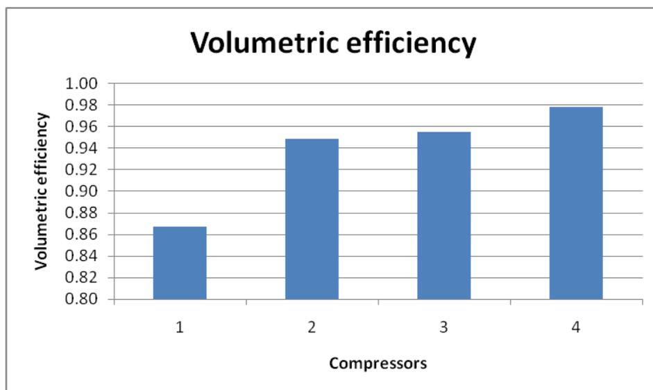
Figure 7: Volumetric Efficiency of Compressors
