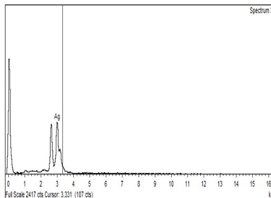
**Figure3. Showing EDX Spectra for Synthesized AgNPs.**
