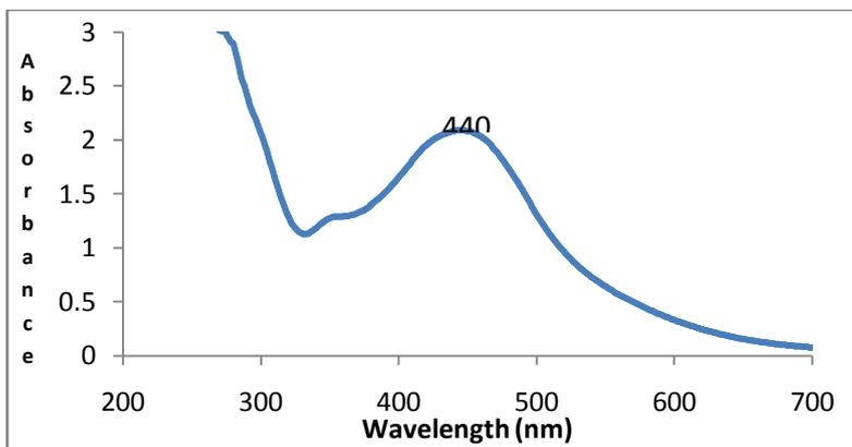
**Figure 1. Showing the UV-visible absorption spectrum of Synthesized AgNPs.**
