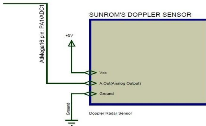
Figure 6. DOPPLER SENSOR INTERFACING WITH ATMEGA16A
