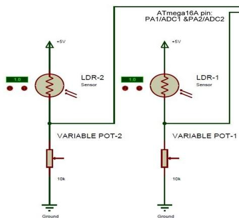
Figure 4. LDR1 & LDR2 INTERFACING WITH ATMEGA16A
