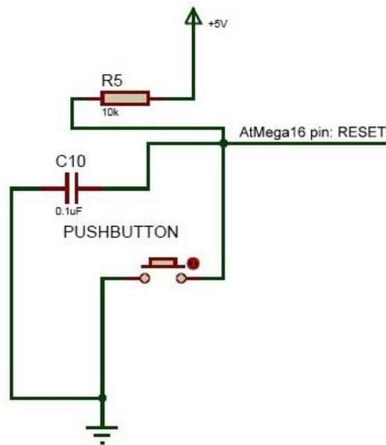
Figure 8. PUSH BUTTON INTERFACING WITH ATMEGA16A
