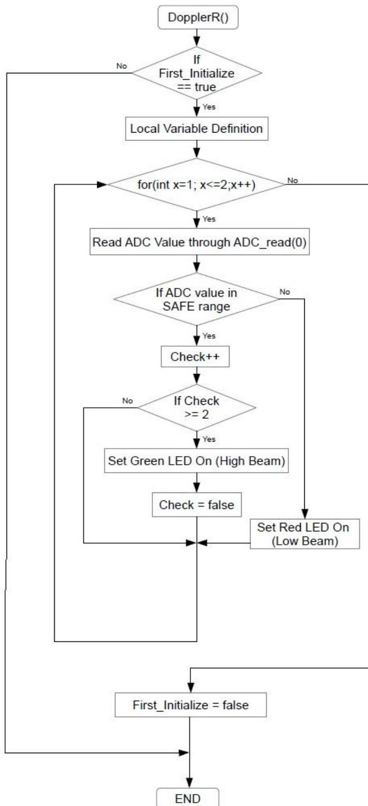
Figure 11. FIRMWARE'S DOPPLERR FUNCTION
