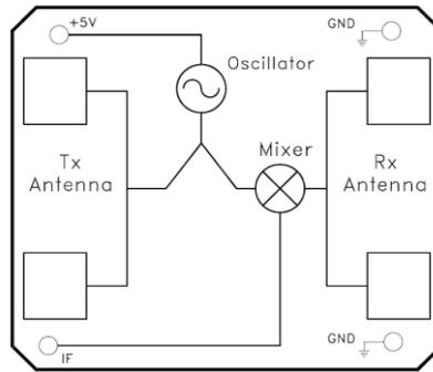
Figure 2. BLOCK DIAGRAM OF SUNROM'S DOPPLER SENSOR (1195) [4]
