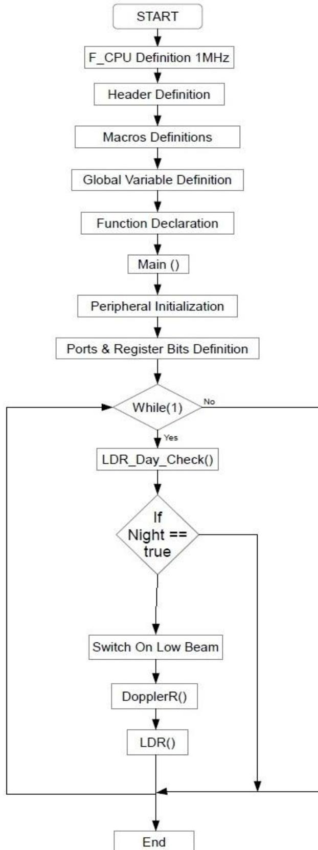
Figure 9. FIRMWARE'S MAIN FUNCTION
