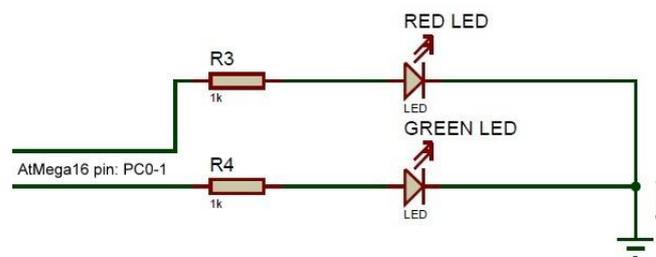
Figure 7. RED & GREEN LED INTERFACING WITH ATMEGA16A
