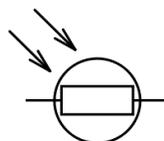
Figure 1. LDR BASIC DIAGRAM
