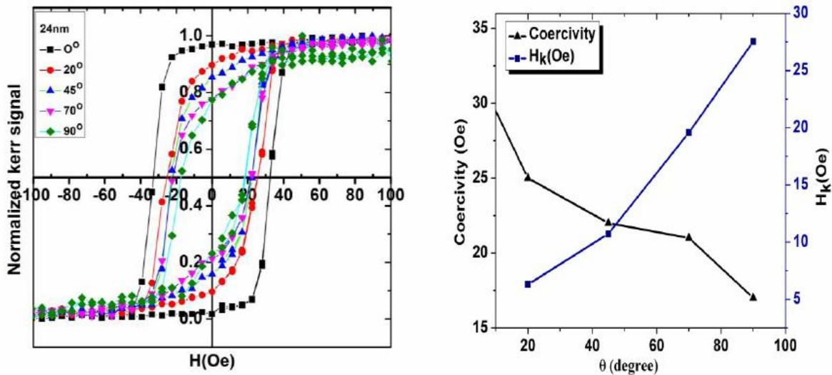
Fig. 5(a) MOKE M-H loops of Si/CoFeB (24nm) film, measured at different angles between applied magnetic field direction and the easy axis.(b) Variation of anisotropy field  $H_k(\theta)$  and coercivity with angle ( $\theta$ ) between easy and hard axis for 300°C annealed CoFeB film (24 nm).
