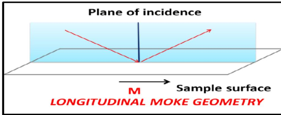
Fig.2 Schematic representation of Longitudinal MOKE (L-MOKE) Geometry
