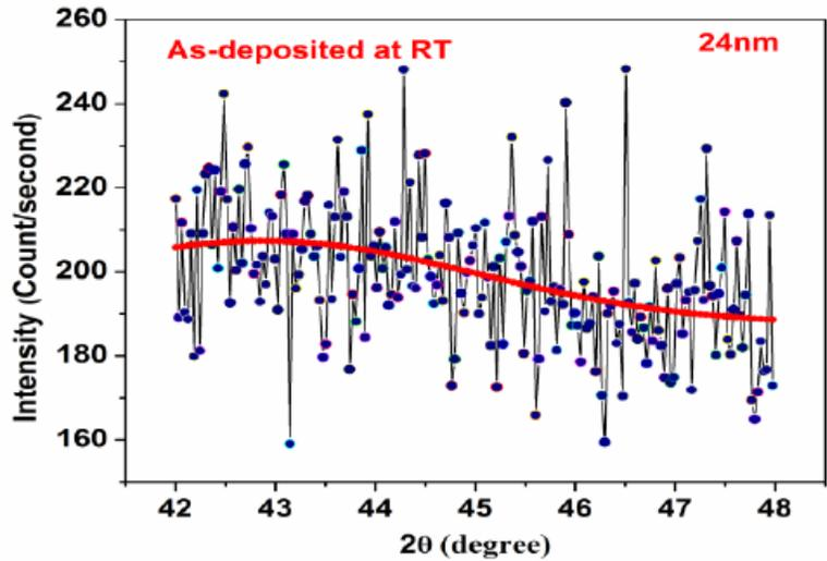
Fig. 1 (a) XRD scan of *as-deposited* CoFeB thin film (24 nm) exhibiting amorphous nature
