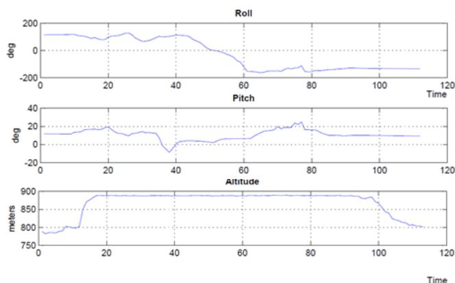
Fig. 7 pitch, roll and altitude from logged data
