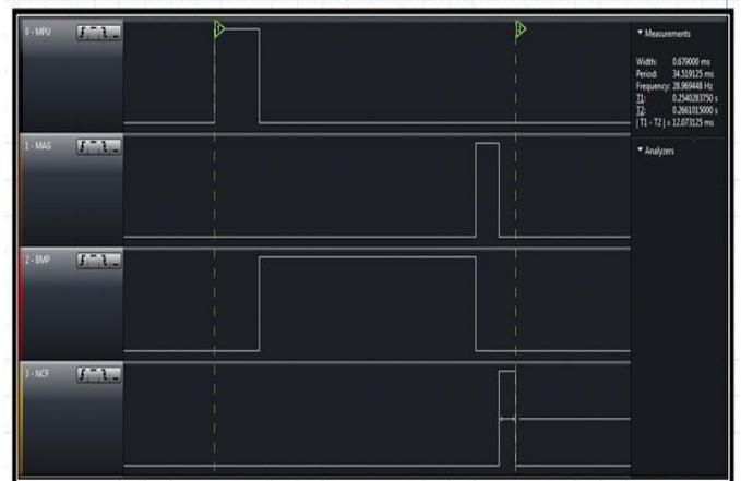
Fig. 6 Execution time for all sensors using Logic Analyzer
