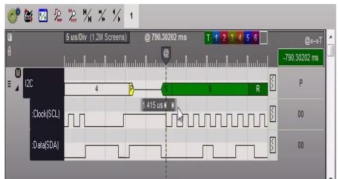
Fig.5 Timing Plot I2C communication shown in logical analyzer
