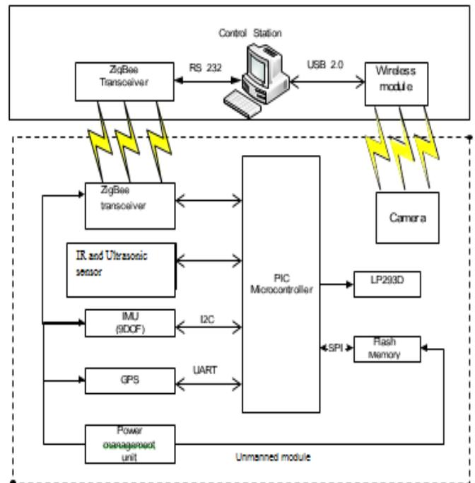
Fig. 1. Autopilot controller board with Control Station
