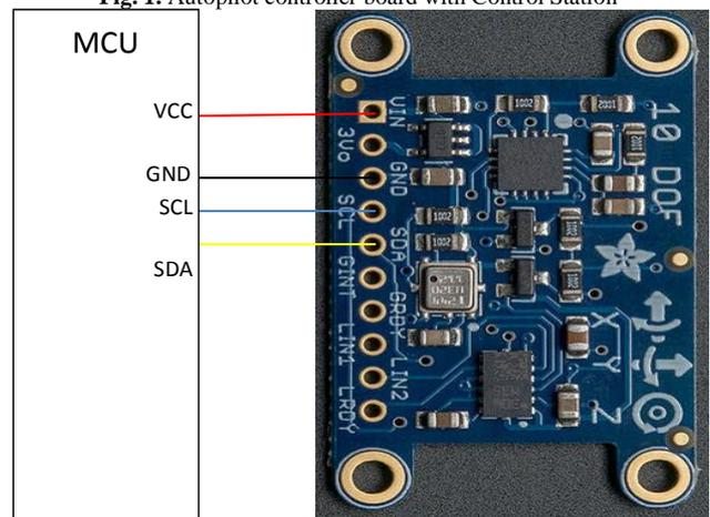
Fig.2 DOF –IMU Sensor Wiring
