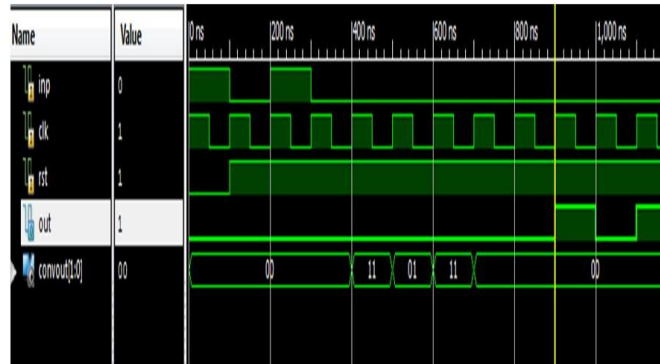
Figure: 15 Simulation result of modified viterbi decoder.
