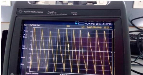
Figure 31 Phase response for Beam forming circuit with array of antennas
