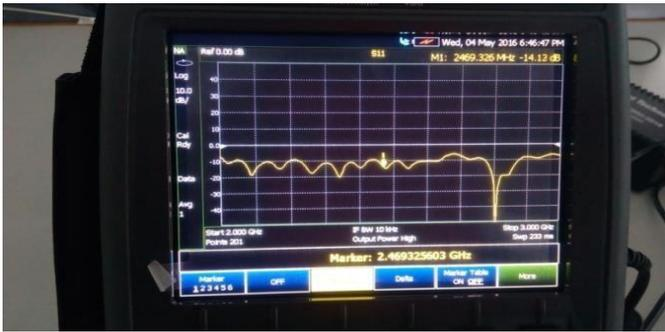
Figure 30 Measurement of S<sub>11</sub> for Beam forming circuit with array of antennas
