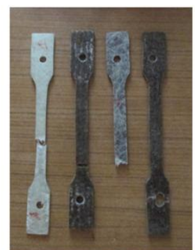
Fig 5.2 After Tensile Testing
