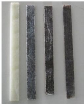
Fig 5.3 Before Flexural Test
